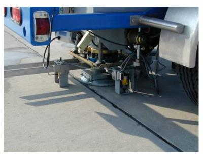
Deflection based LTE (ratio of plastic strains at the two sides of the joints) is the most common method to determine LTE and joint stiffness of PCC slabs in pavement industry.
